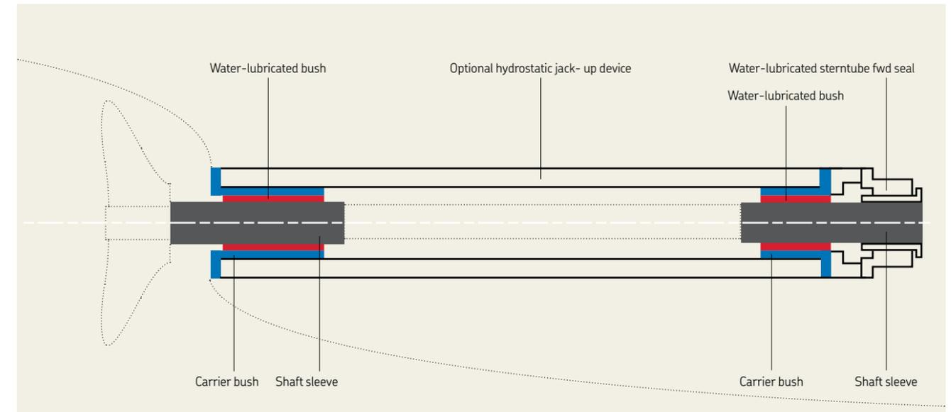
**Type 2: Open water lubricated sterntube system**
