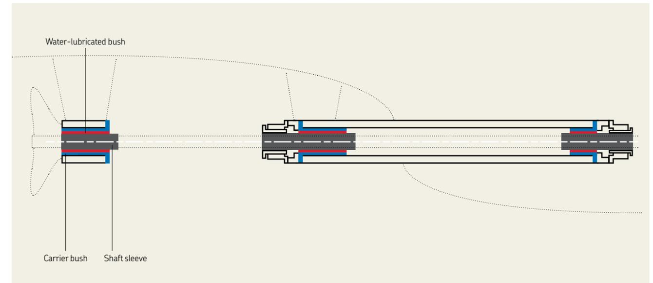
**Type 3: Open sea water-lubricated propeller shaft bearings**
