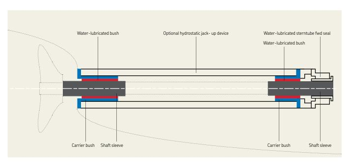
Type 2: Open water lubricated sterntube system
