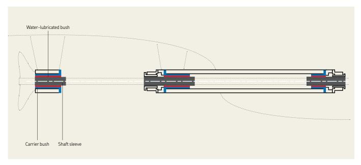
Type 3: Open sea water-lubricated propeller shaft bearings
