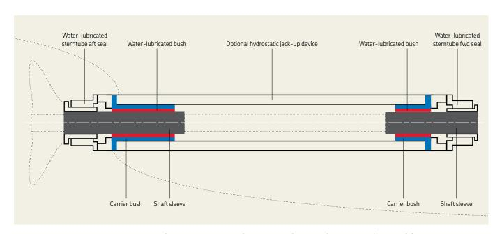
Type 1: Closed sterntube system with fresh water filling and anti-corrosive protection additive
